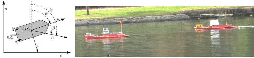
Fig. 2 a) The ASV motion reference model; b) Two vessels during the experiment.
