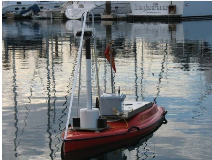
Vertically profiling QBoat can navigate to many parts of harbor to collect data
