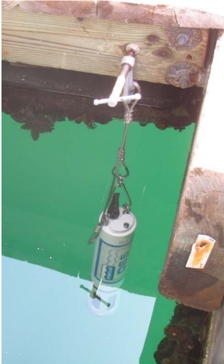
Multi-parameter sondes hung from docks in 3 locations in King Harbor, Redondo Beach
