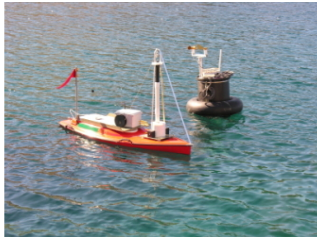
(d) Autonomous Surface Vehicle (ASV) and deployed marina buoy.
